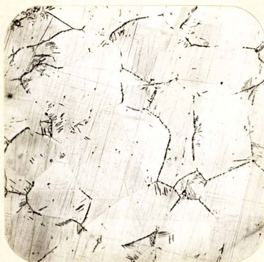
X100, picral etch. AUSTENITIC STRUCTURE WITH FREE CARBIDES ON GRAIN BOUNDARIES AND NEEDLES OF MARTENSITE.
