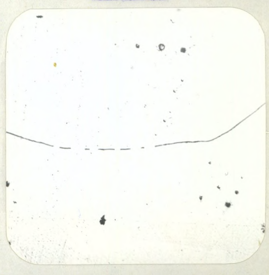
X200, picral etch. SAME AS FIGURE 3. SHOWS DISCONTINUOUS, HEAVY GRAIN BOUNDARIES.
