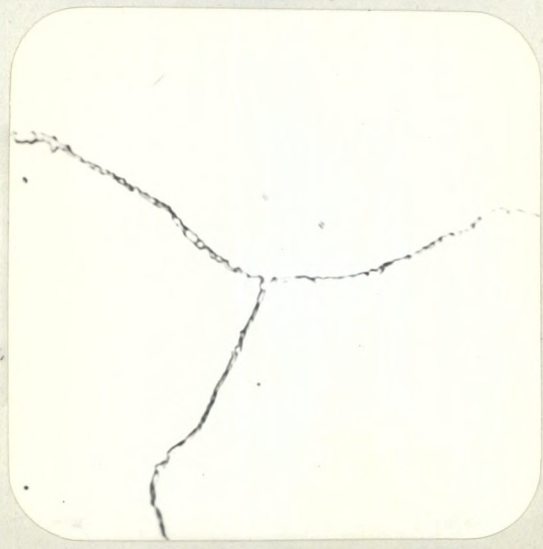
X2000, picral etch. SAME AS FIGURE 5. SHOWS DETAILS OF GRAIN BOUNDARY STRUCTURE.
