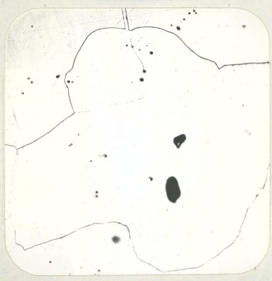
X100, picral etch. PHOTOMICROGRAPH SHOWING STRUCTURE AFTER WATER-QUENCHING PIECE 2" x 2" x 1/2" FROM 1940° F. Note heavy grain boundaries.
