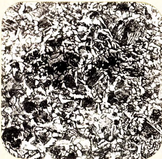
X500, nital etch. CORE STRUCTURE. Low-carbon martensite and ferrite
