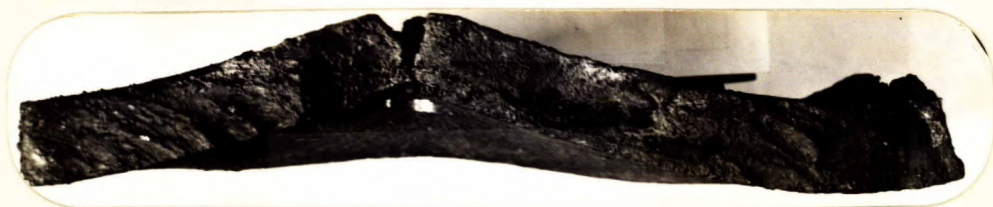
SECTION OF RETORT, SHOWING FAILURE. "AS RECEIVED" CONDITION. (Approximately 1/2 size).
