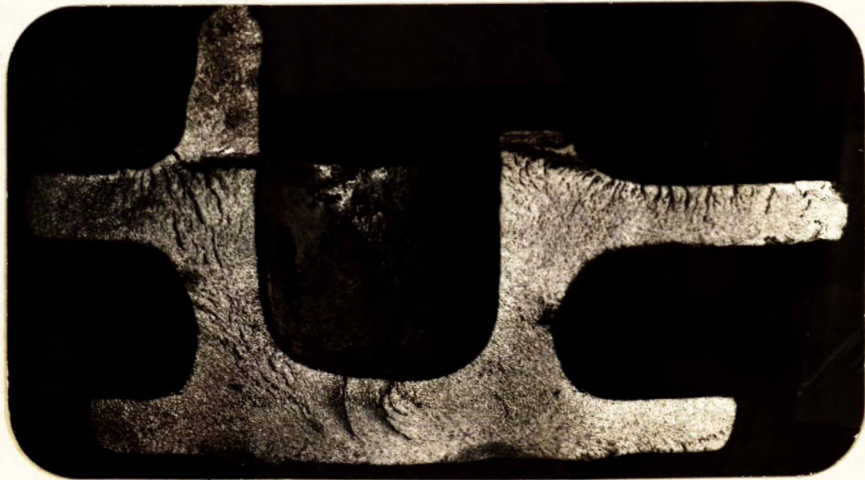
PHOTOGRAPH SHOWING FRACTURE OF CASTING (Approximately 1/3 actual size).
