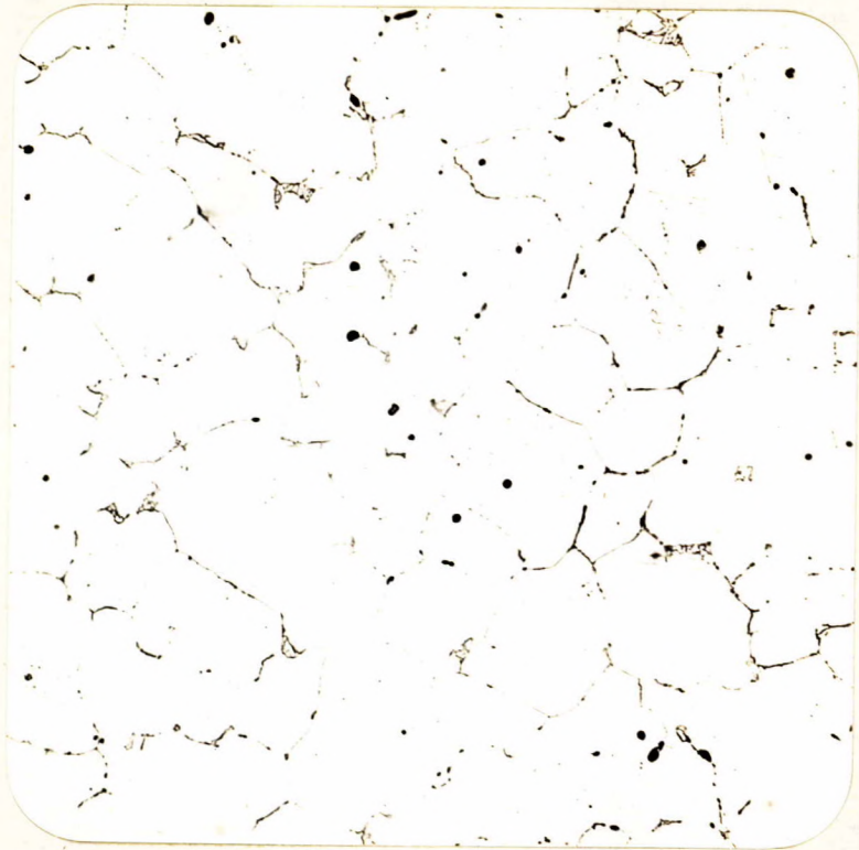
X100, 0.5 per cent HF etch. ARTIFICIALLY AGED MATERIAL.
