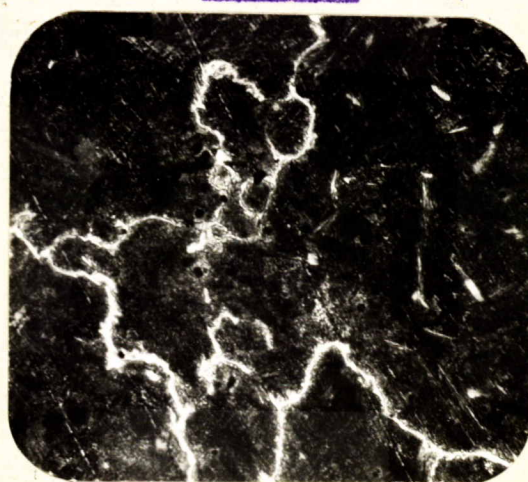
X100, nital etch. McQUAID-EHN AT 2100° F., ROD NO. 2. Grain size: 1-2.
