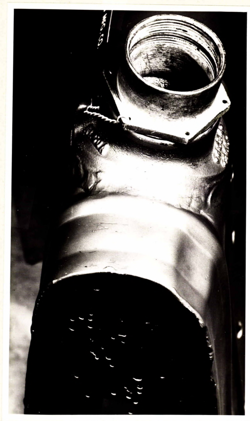
WELD AND AREA OF CORROSION OF DAKOTA PROPELLER DE-ICER TANK.
