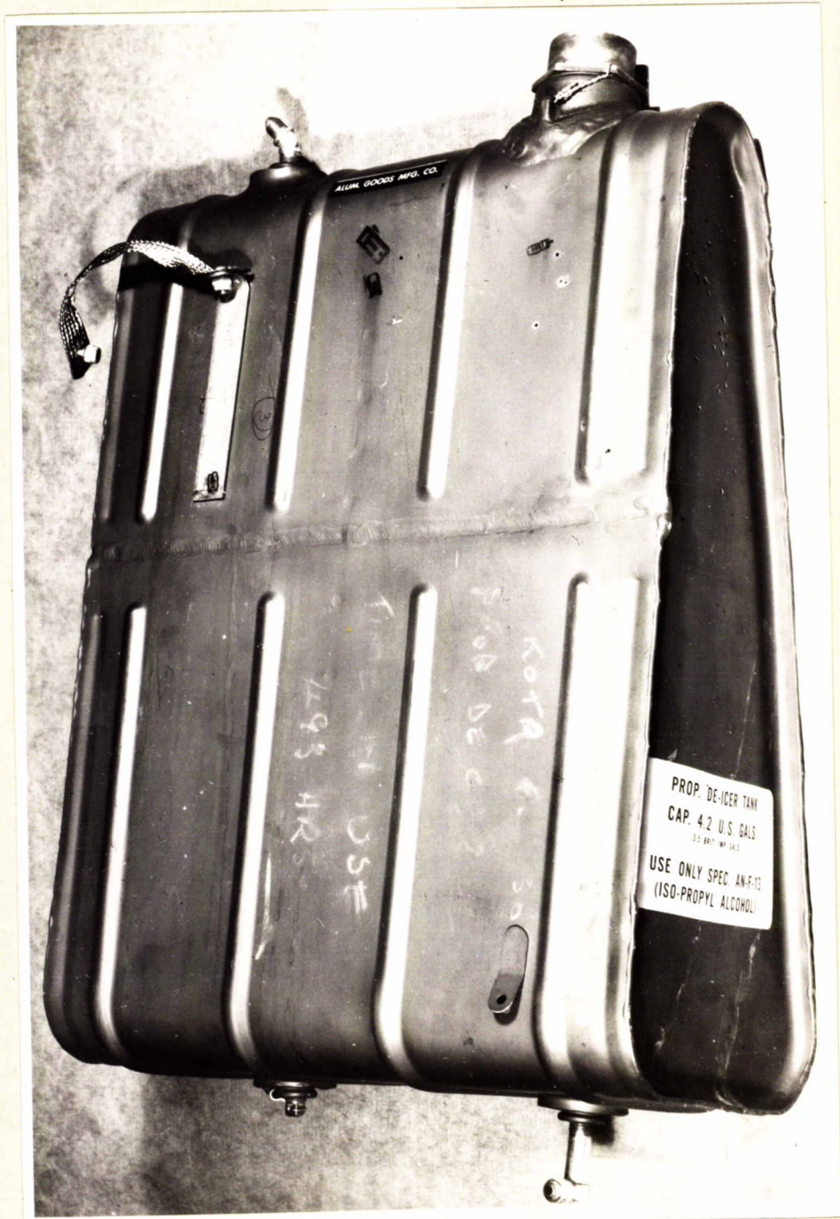
GENERAL SHAPE OF DAKOTA III, F.L. 530, PROPELLER DE-ICER TANK.
