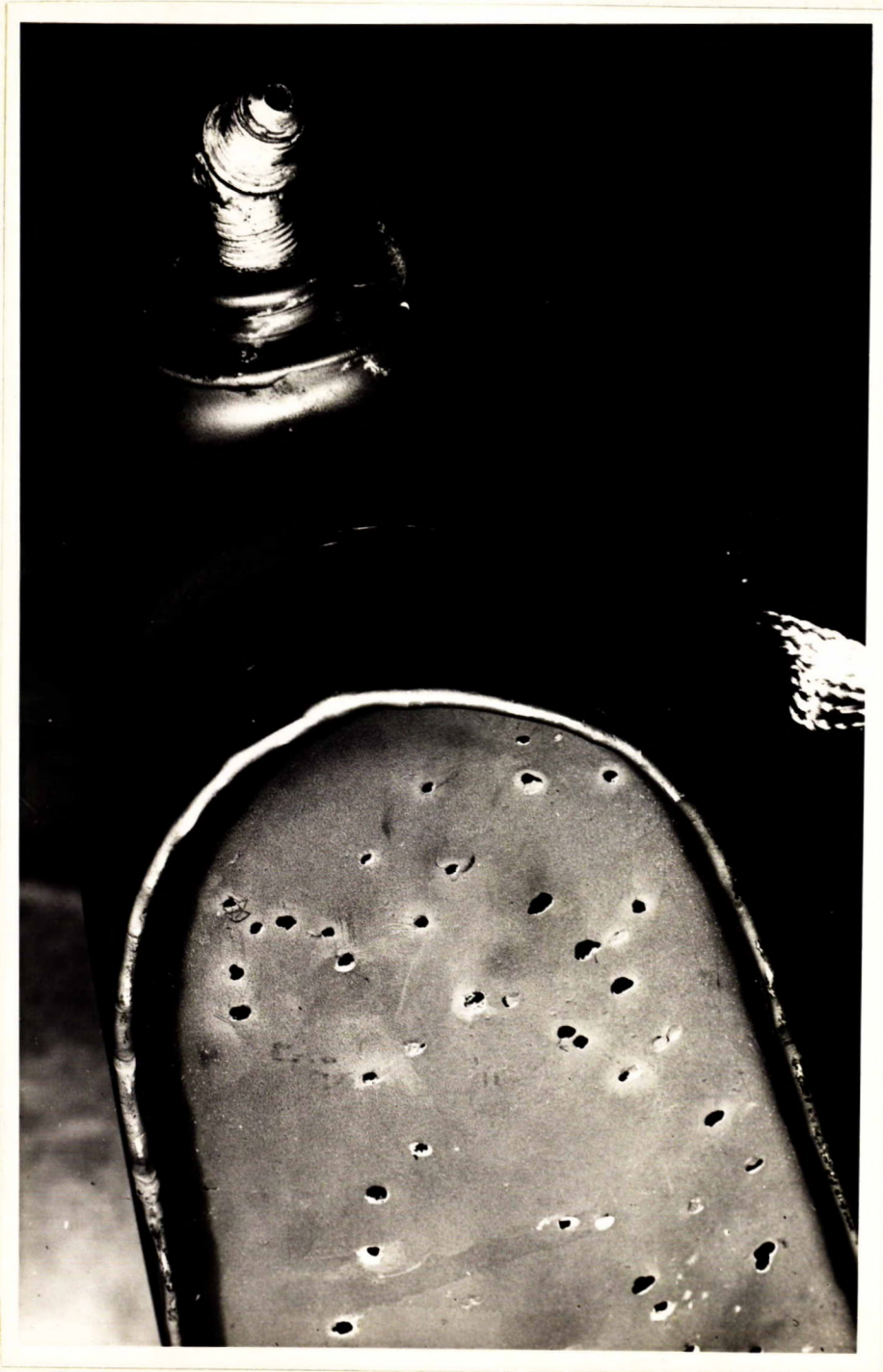
WELD AND AREA OF CORROSION OF DAKOTA PROPELLER DE-ICER TANK.
