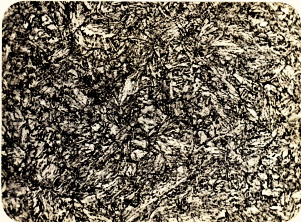
X1500, picral etch. STRUCTURE OF PLATE A (LONGITUDINAL). Tempered martensite.
