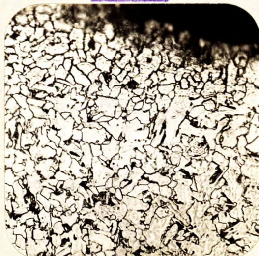
X500, etched in 2 per cent nital. FERRITE AND CARBON-POOR PEARLITE.
