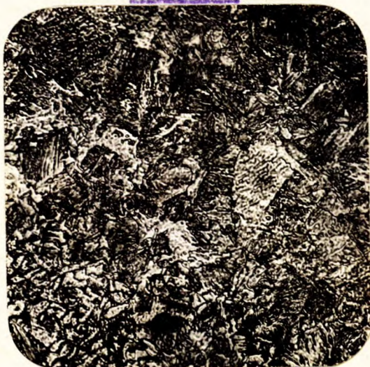
X500, etched in 2 per cent nital. PARTIALLY DECARBURIZED ZONE. Ferrite and low-carbon martensite.
