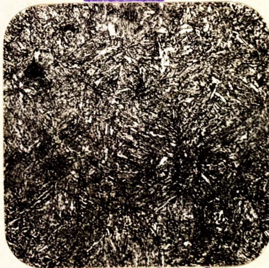
X500, etched in 2 per cent nital. TEMPERED MARTENSITE.
