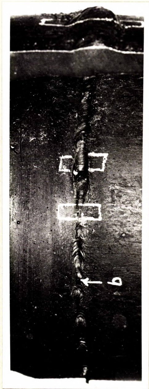
INSIDE OF WELD OF SAMPLE A.
