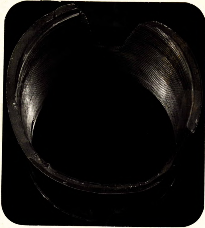
PHOTOGRAPH, ABOUT \frac{1}{2} ACTUAL SIZE, SHOWING FRACTURED PORTION OF PISTON HEAD.
