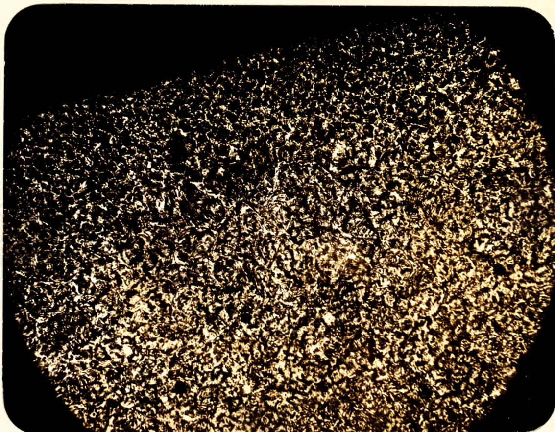
X250, nital etch. SURFACE OF A TIP FROM LOT NO. 1.
