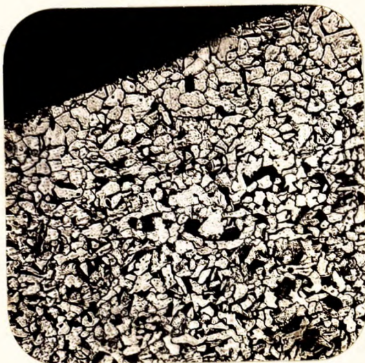
X250, nital etch. SECTION AT SURFACE OF NEW WASHER (SAE 1025).
