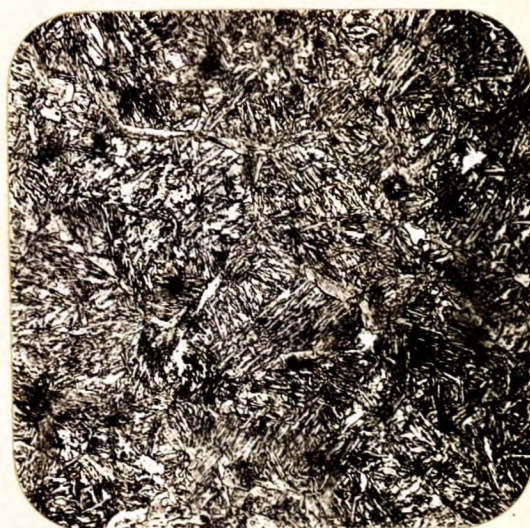
X250, nital etch. STRUCTURE OF HEAT-TREATED WASHER (SAE 1025).
