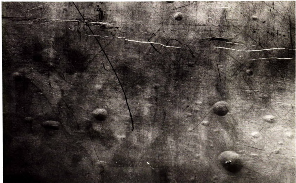
BLISTERED SHEET SAMPLE AS RECEIVED. (Approximately 1\frac{1}{2} times actual size).
