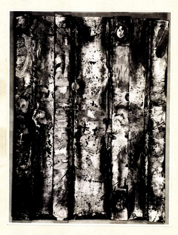
TESTED PLATE AS RECEIVED. White rectangles indicate areas from which micro and macro samples were machined.
