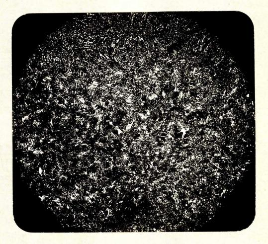
X500, stohed in 2 per cent nital. TYPICAL STRUCTURE OF TRANSITION ZONES OF ALL WELDS.
