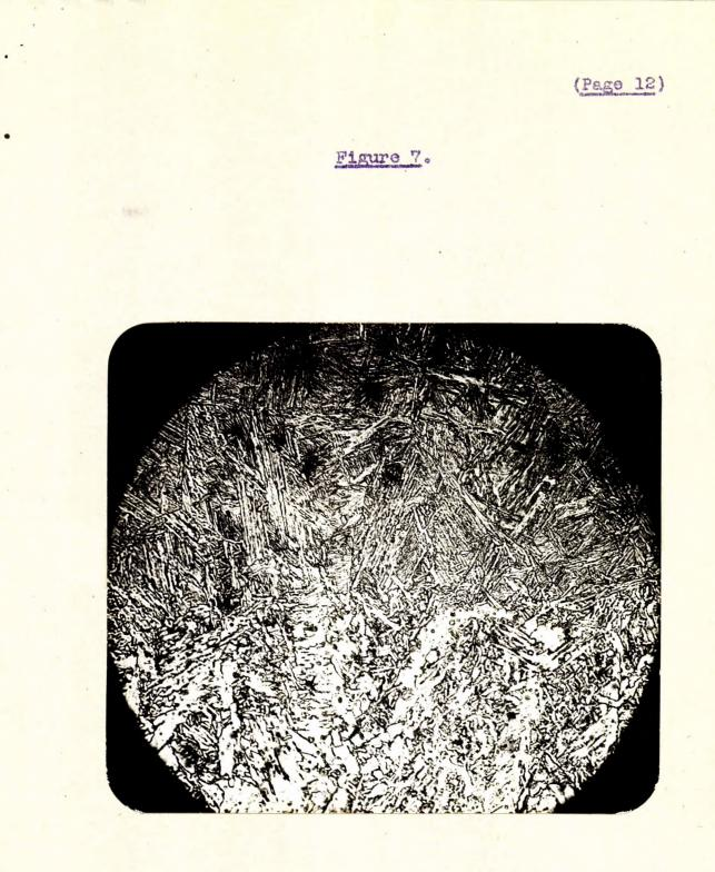
X500, etched in 2 per cent nital. TYPICAL FUSION ZONE OF A FERRITIC WELD.
