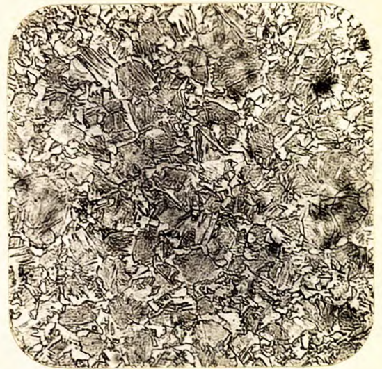
X500, nital etch. CORE OF PIN NO. 8.
