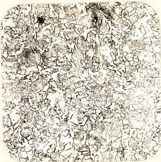
X500, nital etch. CORE OF PIN NO. 9.
