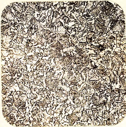
X500, nital etch. CORE OF PIN NO. 2.
