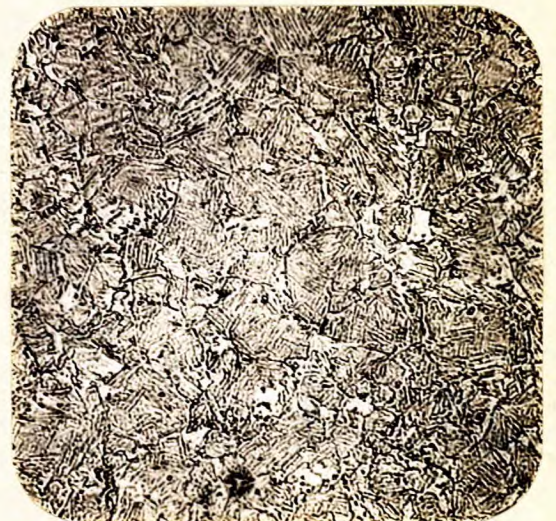
X500, nital etch. CORE OF ALLIED PRODUCTS PIN.
