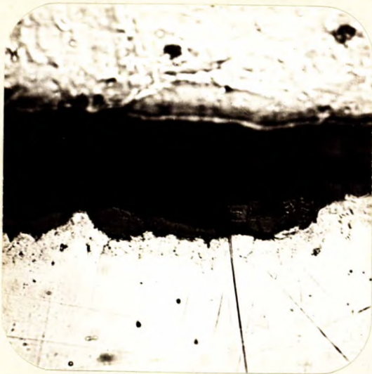
X500, unetched. SHOWING THE EXTENT OF SCALING.
