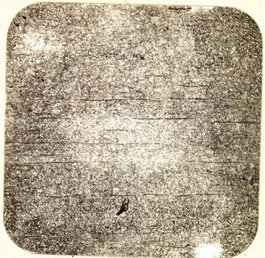
X100, picral etch. SHOWING AN INCLUSION PATTERN.
