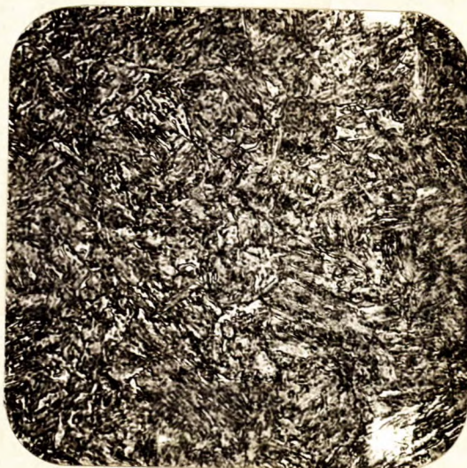
X500, picral etch. SHOWING THE MICROSTRUCTURE OF THE STEEL.
