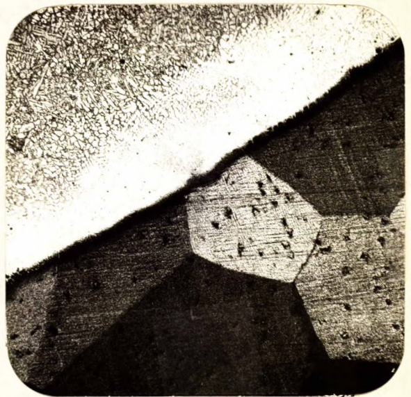
X100, FeCl 3 etch. BRAZED JOINT.
