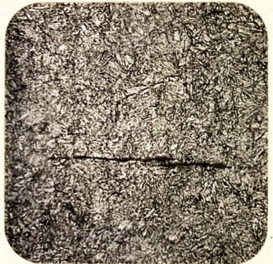
X500, picral etch, SHOWING THE MICROSTRUCTURE OF AEDB LOT NO. 818.
