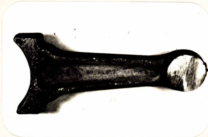
FORGING "AS RECEIVED". (Approximately 3/8 size).
