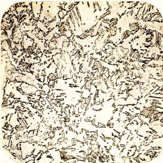
X500, nital etch. TYPICAL CORE OF MATILDA PIN.
