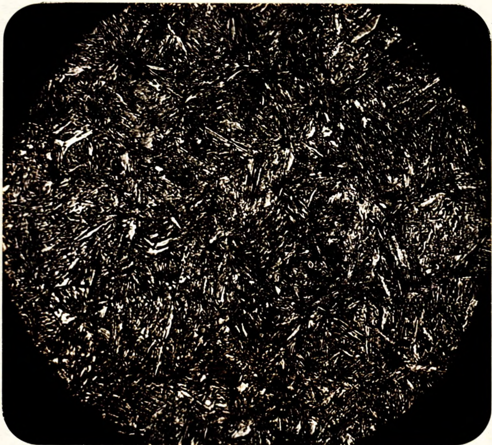
X1000, nital etch. CASE STRUCTURE OF CHURCHILL PIN.
