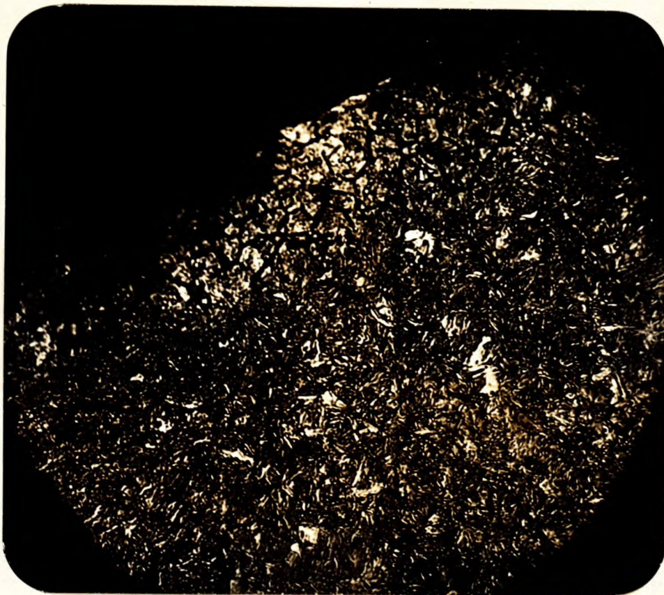
X1000, nital etch. CASE STRUCTURE OF UNIVERSAL CARRIER PIN. Note black constituent outlining grain boundaries at surface.
