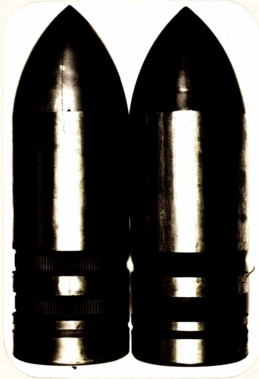
PHOTOGRAPH OF SHOT, DEPICTING "TYPICAL" CRACKS.
