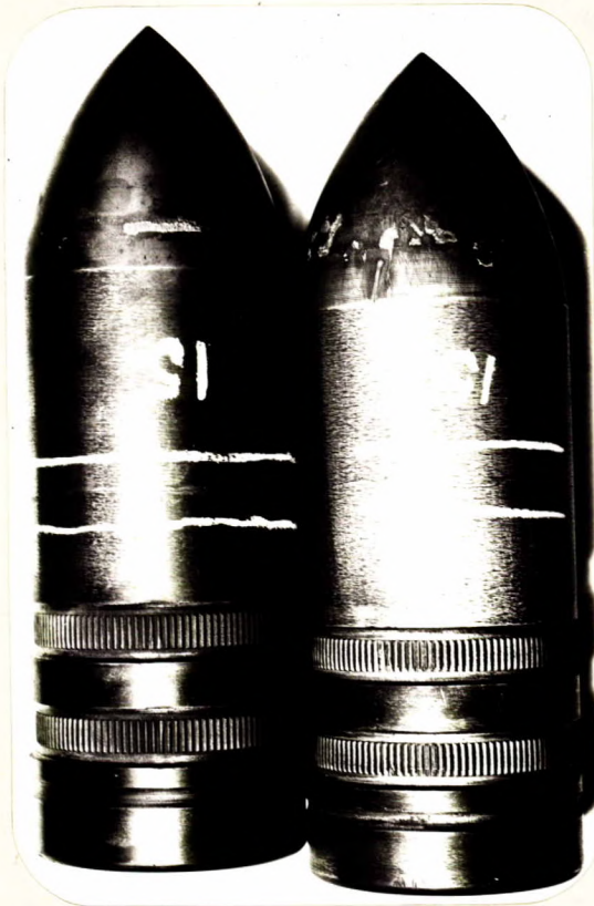
CIRCUMFERENTIAL CRACKS DEVELOPED BY 1:1 HCl ETCHING FOR 15 MINUTES.
