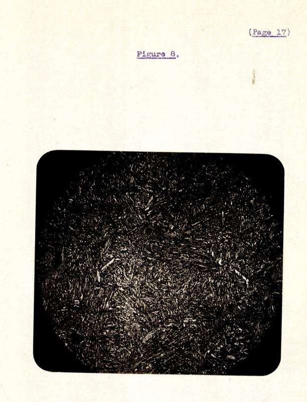
X500, etched in 4 per cent picral, NORMAL PLATE STRUCTURE OF TEMPERED MARTENSITE.
