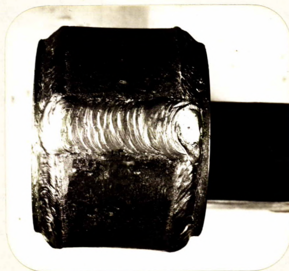
PHOTOGRAPH OF WELD JOINING ENDS OF STRAP MATERIAL.
