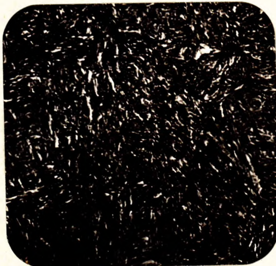
X1000, nital etch. TEMPERED MARTENSITE.
