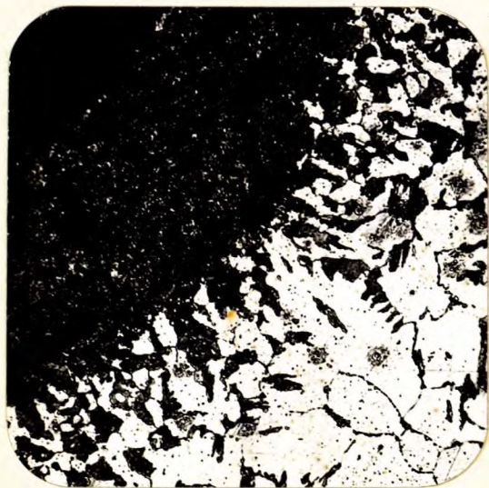
X200, nital etch. AUSTEMPERED LINK, CYANIDE CASE.
