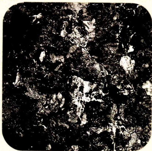
X200, nital etch. BLACKHEART MALLEABLE, CORE STRUCTURE.
