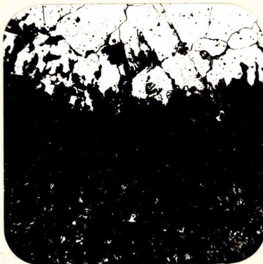
X200, nital etch. BLACKHEART MALLEABLE, CYANIDE CASE.
