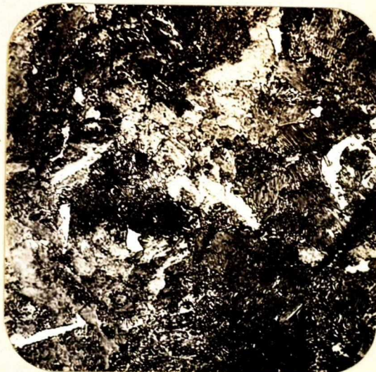
X500, nital etch. AUSTEMPERED MALLEABLE, CORE STRUCTURE.
