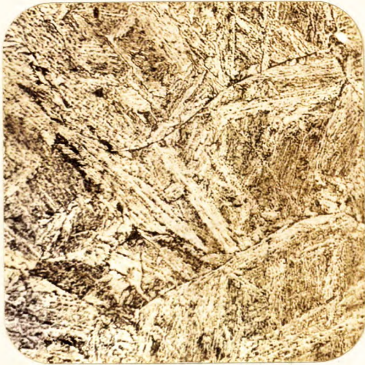
X500, picral etch. HEAT-AFFECTED ZONE IN SPONSON PLATE NO. 3.
