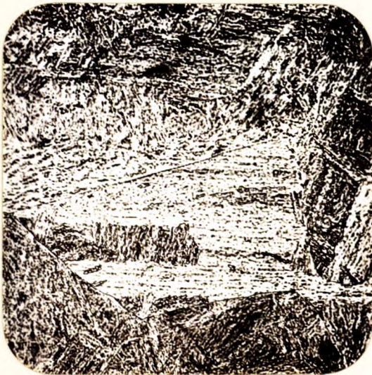
X500, picral etch. HEAT-AFFECTED ZONE IN SIDE PLATE NO. 2.
