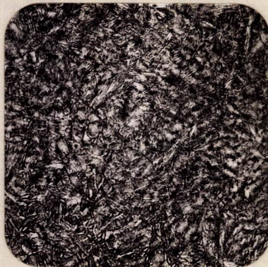
X500, picral etch. NORMAL STRUCTURE IN SIDE PLATE NO. 1.
