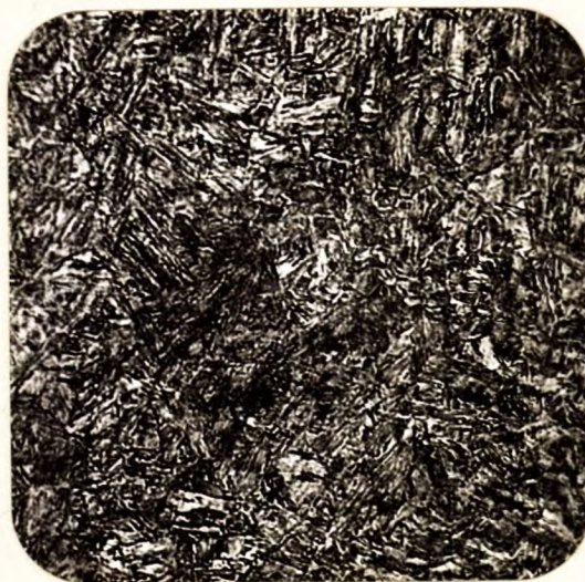
X500, picral etch. NORMAL STRUCTURE IN SIDE PLATE NO. 2.
