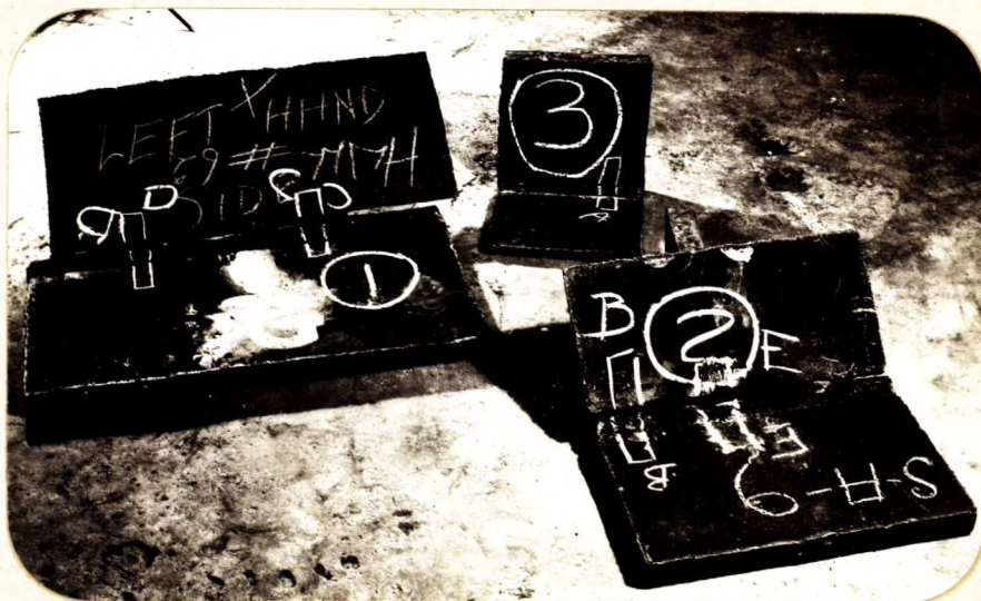
SHOWING THE THREE WELDED SPECIMENS "AS RECEIVED" AND THE LOCATION OF SECTIONS TAKEN FOR EXAMINATION.
