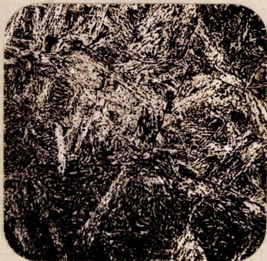
X500, picral etch. HEAT-AFFECTED ZONE IN SIDE PLATE NO. 3. -
