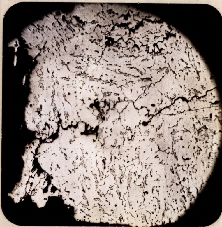
X42. Etch, 0.15 per cent HF in water. CRACK IN EXHAUST PORT.
