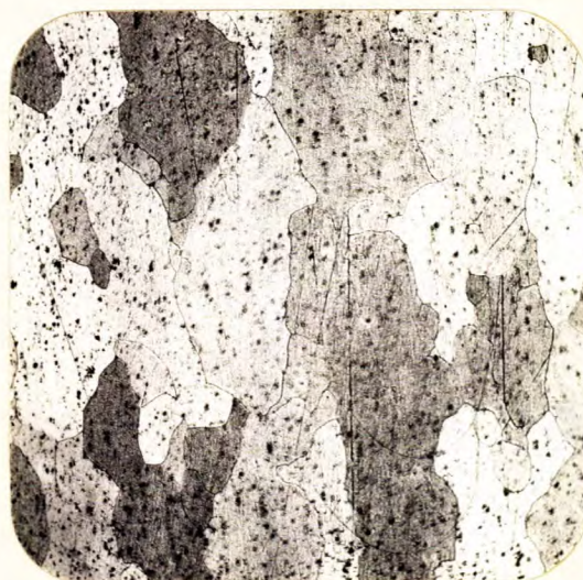
X100, Keller's etch. SAMPLE 1, TYPE 4 RIVET.
