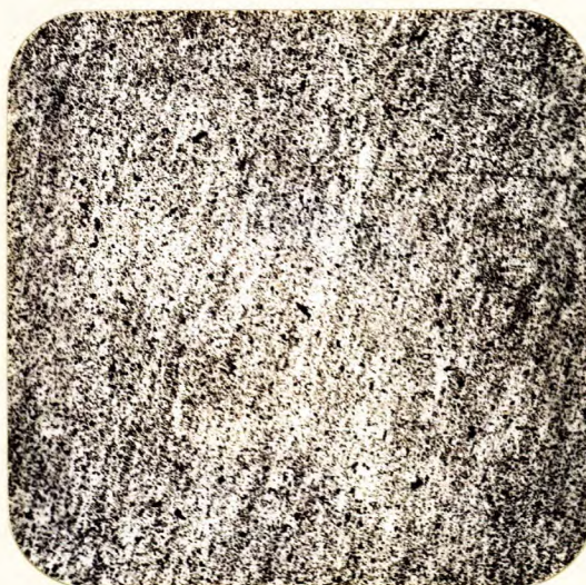
X100, Keller's etch. SAMPLE 3, TYPE 4 RIVET.
