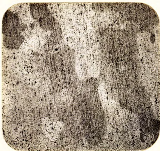
X100, Keller's etch. SAMPLE 2, TYPE 4 RIVET.
