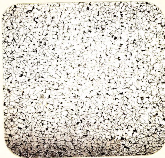
X100, etched in 2 per cent nital. STRUCTURE \frac{1}{2} INCH FROM FRACTURE.
