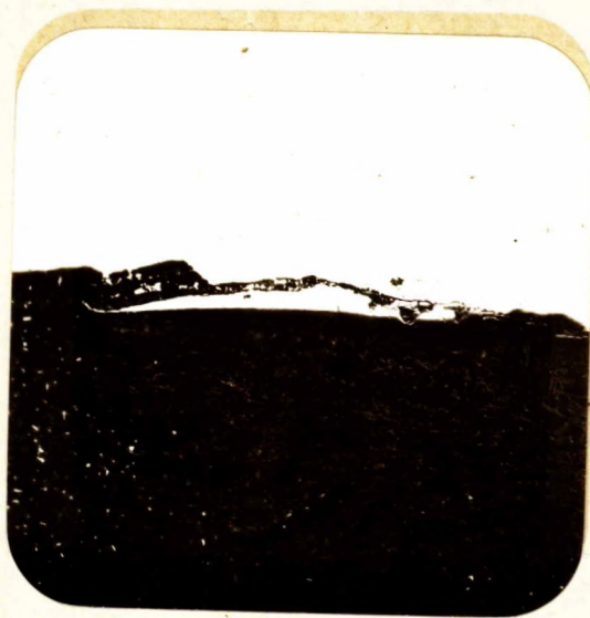
PHOTOMICROGRAPH, X100, UNETCHED, SHOWING CROSS-SECTION OF SURFACE OF SHELL ON LEFT-HAND SIDE OF FIGURE 1 AT LINE OF SURFACE CRACKS.
