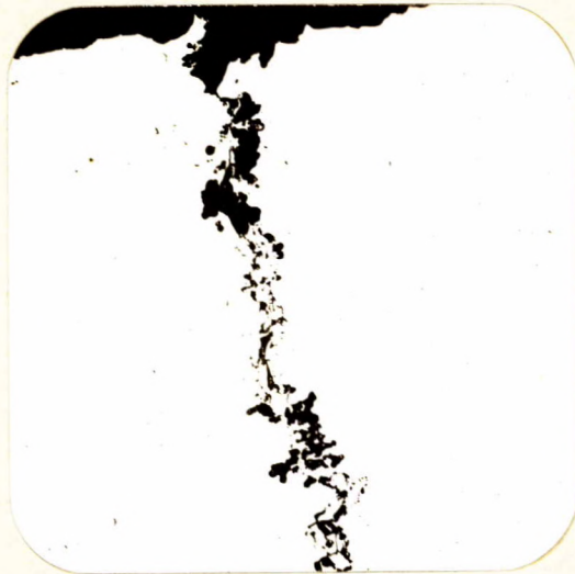
PHOTOMICROGRAPH, X100, UNETCHED, SHOWING A TRANSVERSE SECTION OF A CRACK.
