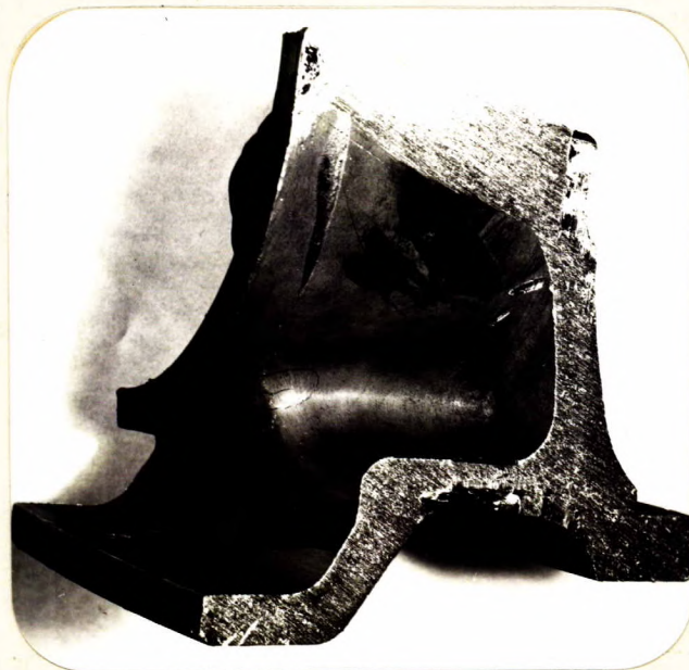
CRACK IN FORGED CRANKCASE. (Approximately 1/2 size).
