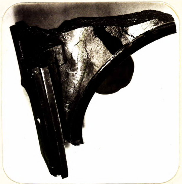
CRACKS IN CAST CRANKCASE. (Approximately 1/2 size).
