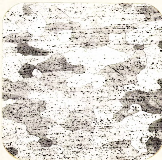
X100, Keller's etch. BODY OF RIVET FROM BOX NO. 5.
