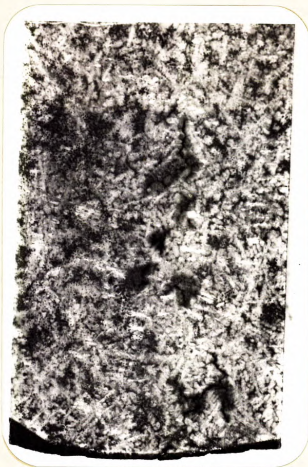
X3, etched in 50 per cent hydrochloric acid. LIGHT DEEP-ETCHED SECTION, HALF-WAY TO CENTRE. Note numerous intercrystalline cracks.
