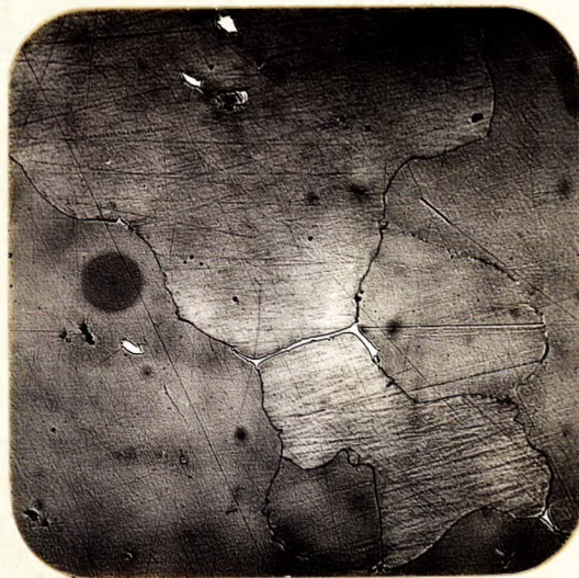
X100. Nital Etched. Grouser Section. (Note free carbides-white constituent)
