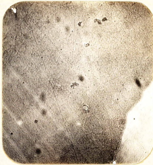
X500. Nital Etched. Rib Section. (Note showing of free carbides at two points)
