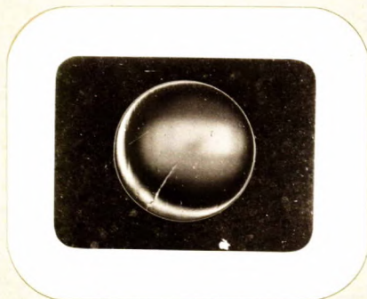
CROSS-SECTION OF CRACKED ROD. (Approximately actual size).
