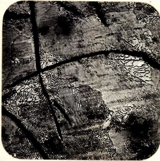
X500, picral etch. PHOTOMICROGRAPH, A.E.D.B. LOT NO. 459B.
