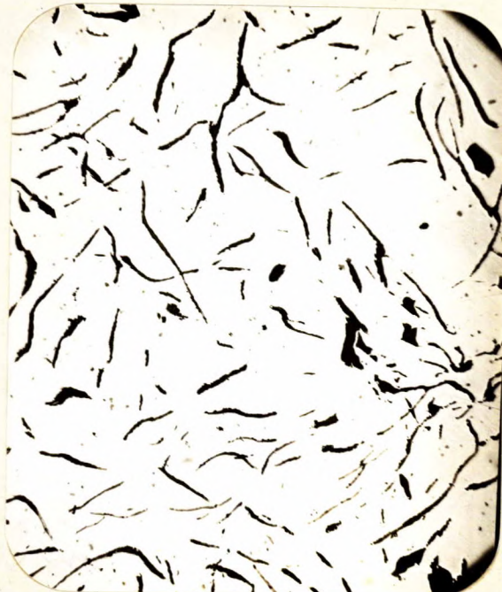
X100, unetched. PHOTOMICROGRAPH, A.E.D.B. LOT NO. 453A, SHOWING GRAPHITE.
