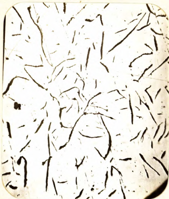
X100, unetched. PHOTOMICROGRAPH, A.E.D.B. LOT NO. 452B, SHOWING GRAPHITE.
