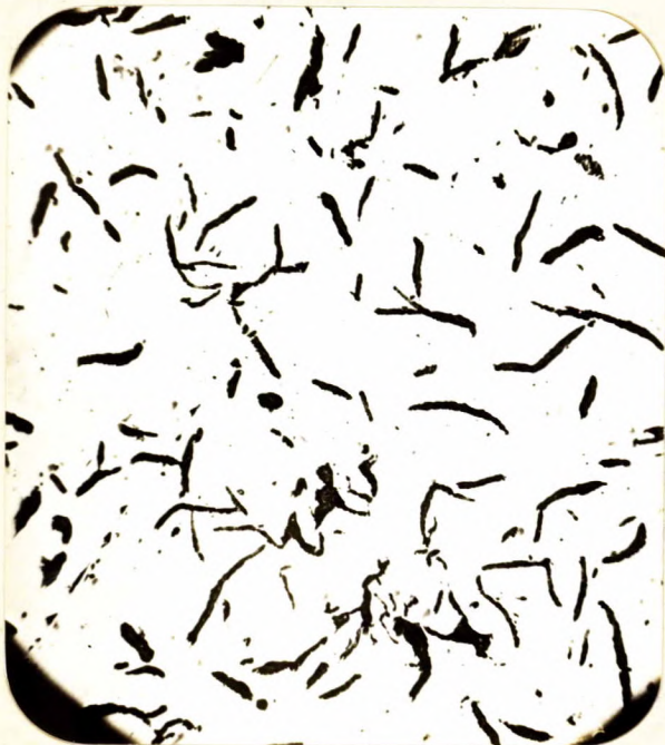
X100, unetched. PHOTOMICROGRAPH, A.E.D.B. LOT NO. 458A, SHOWING GRAPHITE.
