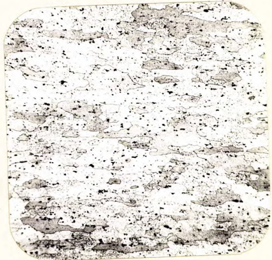
X100, Keller's etch. TRANSVERSE SECTION.
