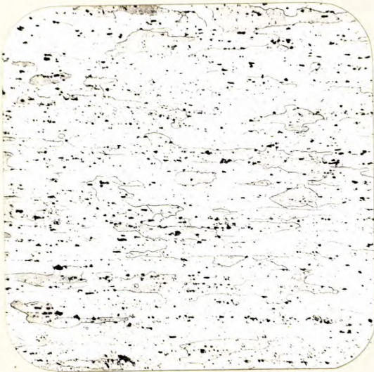
X100, Keller's etch. LONGITUDINAL SECTION.
