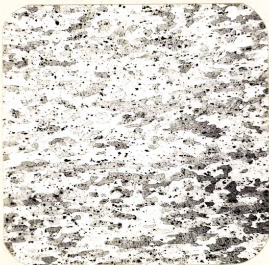
X100, Keller's etch. LONGITUDINAL SECTION.
