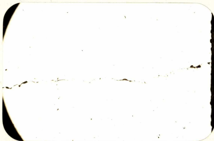
X100, unetched. CROSS-SECTION OF THE DEFECT.
