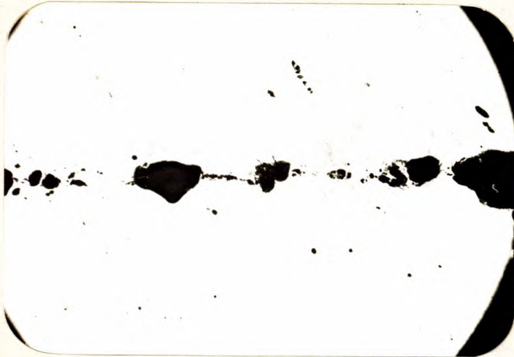
X100, unetched. POROUS METAL.
