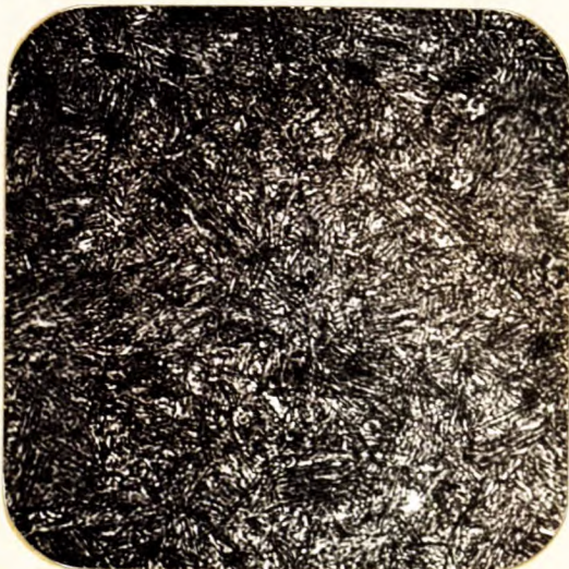
500X, etched in 2 per cent nital. CORE STRUCTURE - TEMPERED MARTENSITE.
