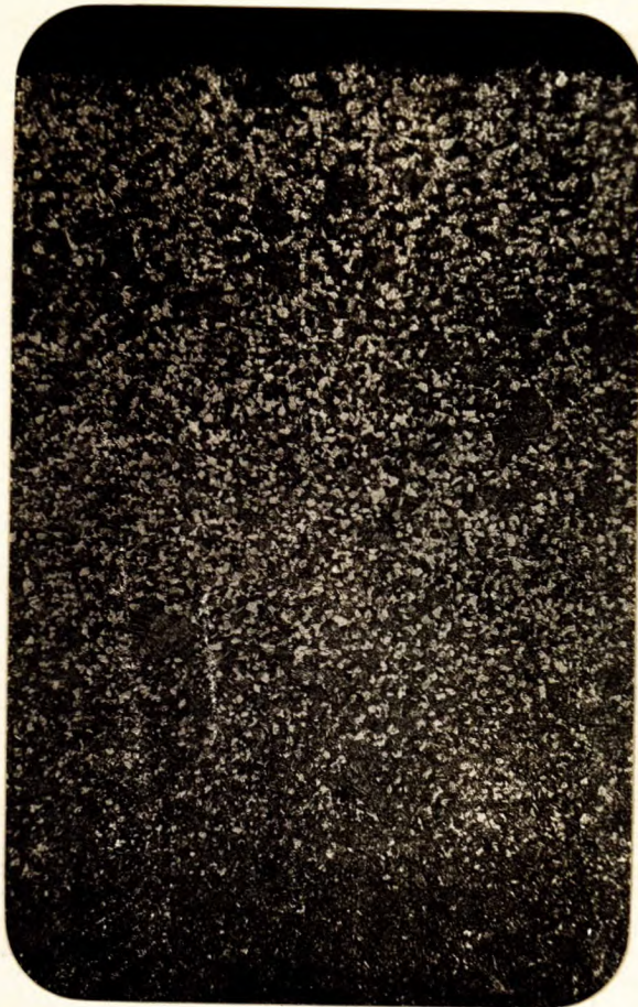
75X, etched in 2 per cent nital. STRUCTURE FROM SURFACE TOWARDS CORE.
