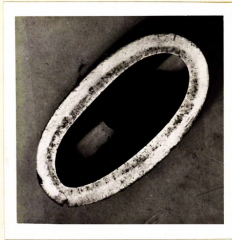
PHOTOGRAPH OF MACRO-ETCHED SECTION FROM PAGE HERSEY TUBE WHICH CRACKED IN FLATTENING TESTS. (Approximately twice actual size).
