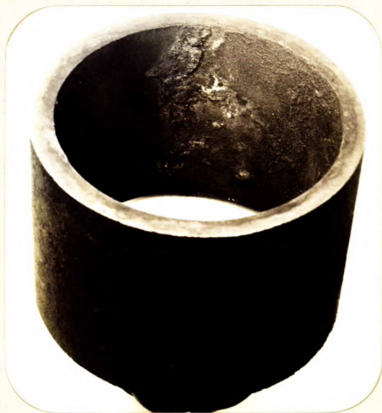
SHOWING SCALE ON INNER SURFACE OF TUBE.
