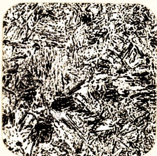
X1000, nital etch. OIL-QUENCHED PIN.
