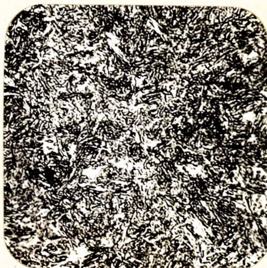
X1000, nital etch. WATER-QUENCHED PIN.
