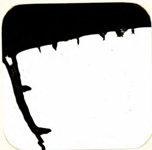
BARREL NO. L21668 CROSS-SECTION OF ERODED SURFACE, TAKEN ABOUT 2 INCHES FROM COMMENCEMENT OF RIFLING.
