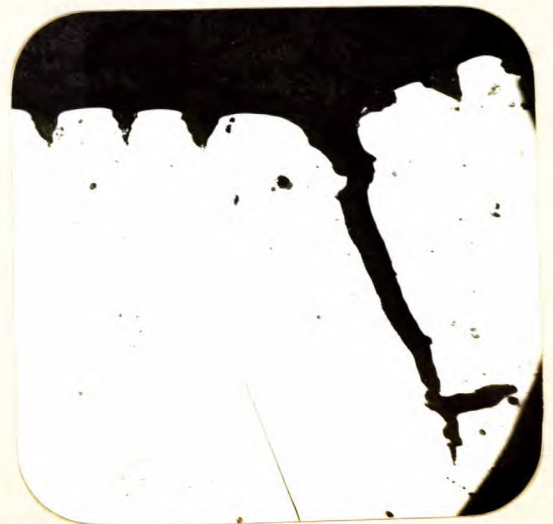
BARREL NO. L21812. CROSS-SECTION OF ERODED SURFACE, TAKEN ABOUT 2 INCHES FROM COMMENCEMENT OF RIFLING.
