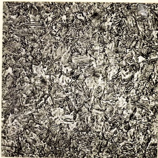
X500, nital etch. CORE OF PIN.
