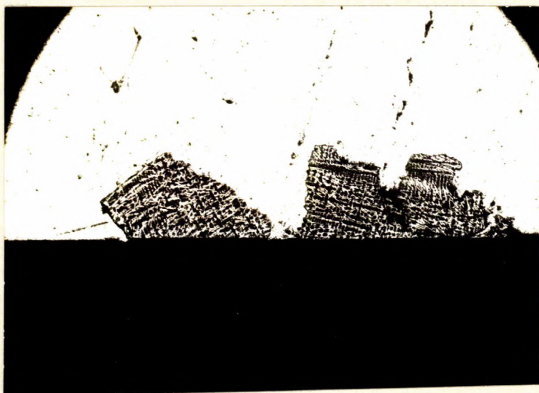
X100, etched in 2 per cent nital. PHOTOMICROGRAPH SHOWING PARTICLES OF WHITE IRON SHOT EMBEDDED IN ALUMINIUM ALLOY PISTON.
