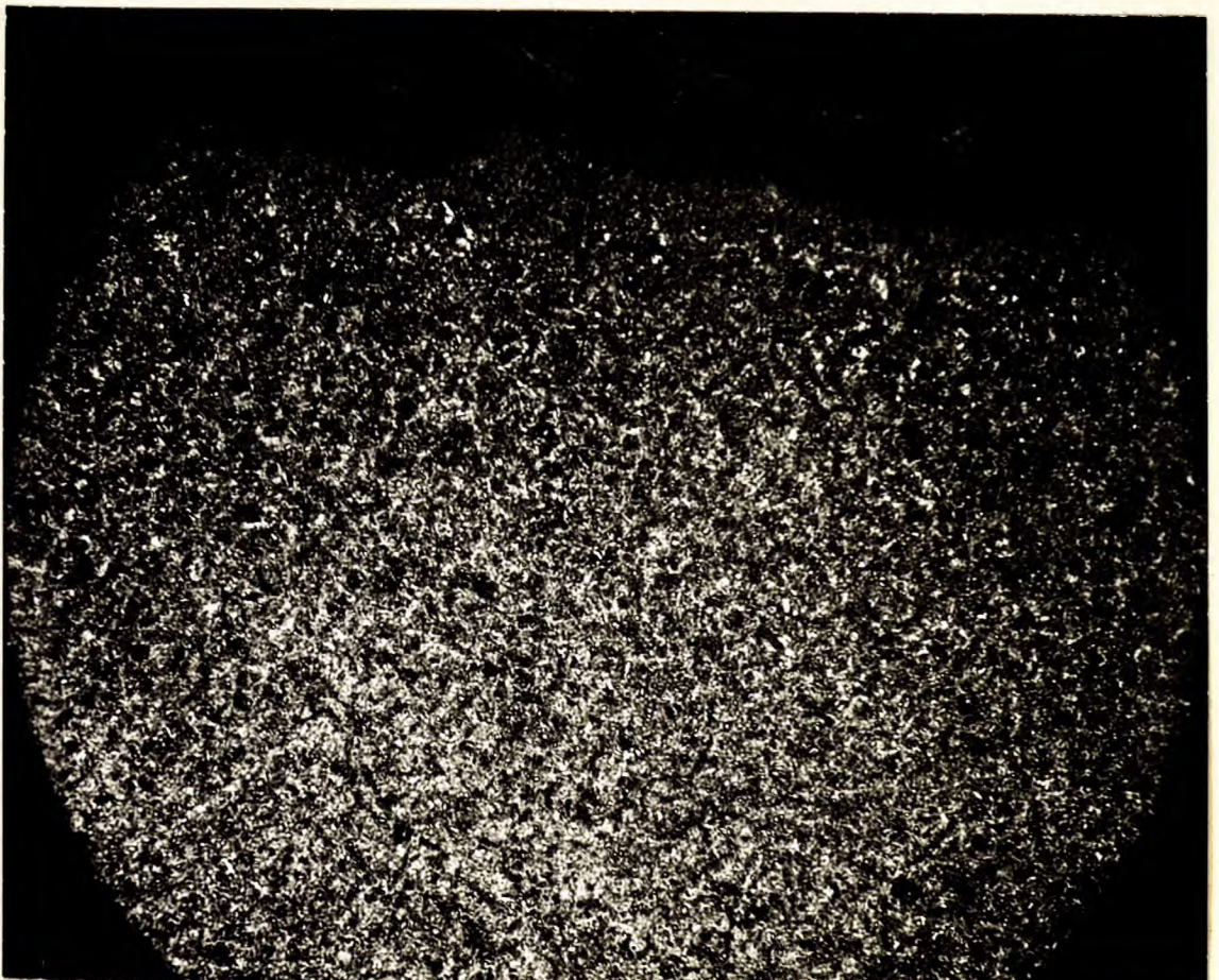
X250 nital etch. 75 MINUTES IN CYANIDE BATH.
