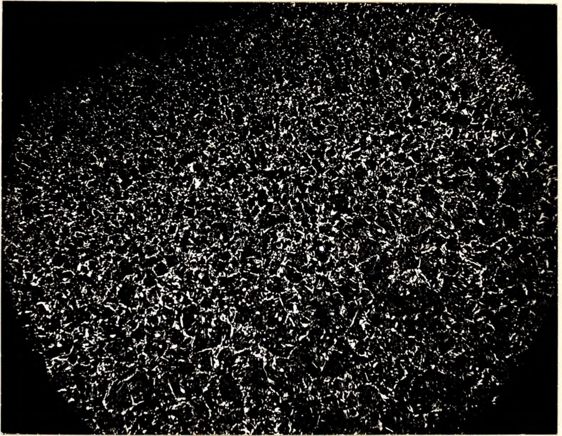
X250, nital etch. 60 MINUTES IN CYANIDE BATH. Note ferrite at grain boundaries.
