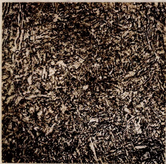
X500, nital etch. STRUCTURE OF SQUARE IMPACT SPECIMEN FROM HEAT B3604.
