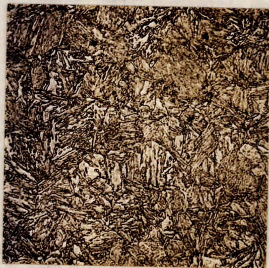
X500, nital etch. STRUCTURE OF SQUARE IMPACT SPECIMEN FROM HEAT OF A3618.
