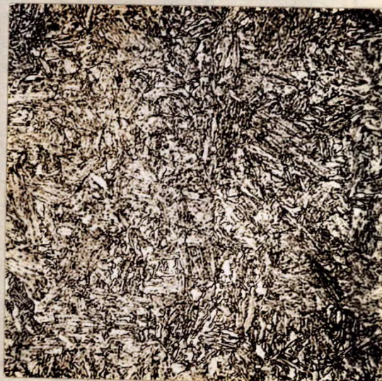
X500, nital etch. STRUCTURE OF SQUARE IMPACT SPECIMEN FROM HEAT A3222.
